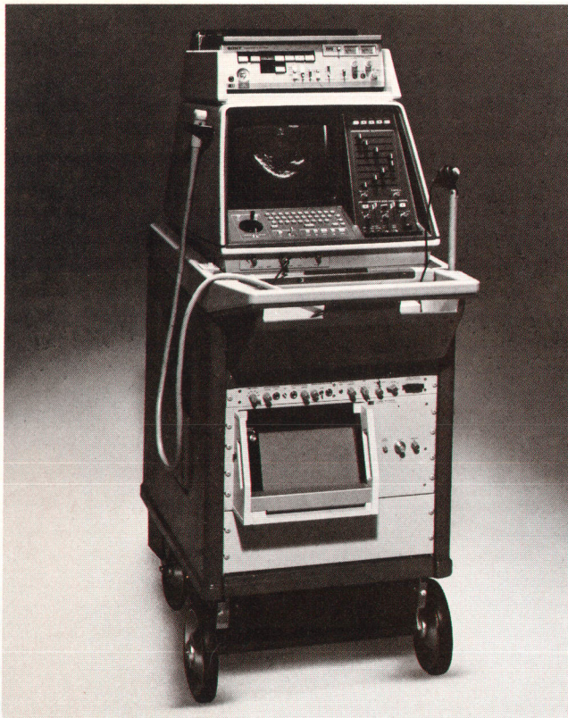
Fig. 1. HP Model 77020A Ultrasound Imaging System provides both M-mode and two-dimensional sector scans of human tissue for cardiac, obstetric, and abdominal examinations. The system is mounted on a mobile cart in a configuration for rapid and easy use.
